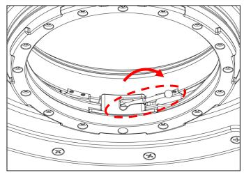
Turn the locking device sideways into the recess. Ensure that the locking device is secured inside the recess and the extension ring is securely locked with the port.
